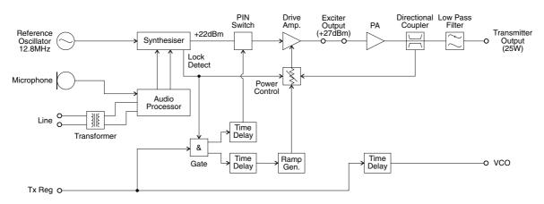
Figure 2.1 T836 High Level Block Diagram
