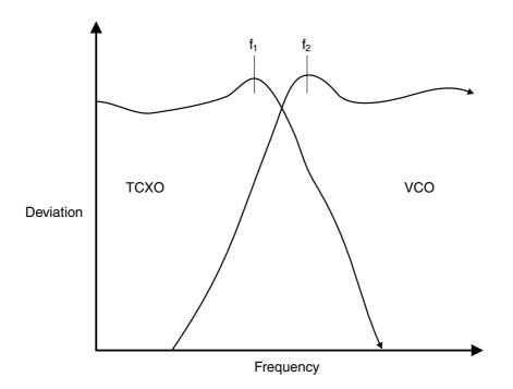
Figure 2.5 T836/837 Two Point Modulation
