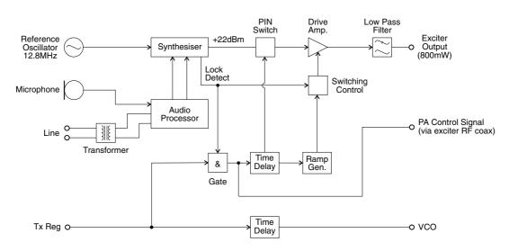
Figure 2.2 T837 High Level Block Diagram
