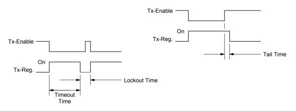
Figure 2.8 T836/837 Transmit Timers
