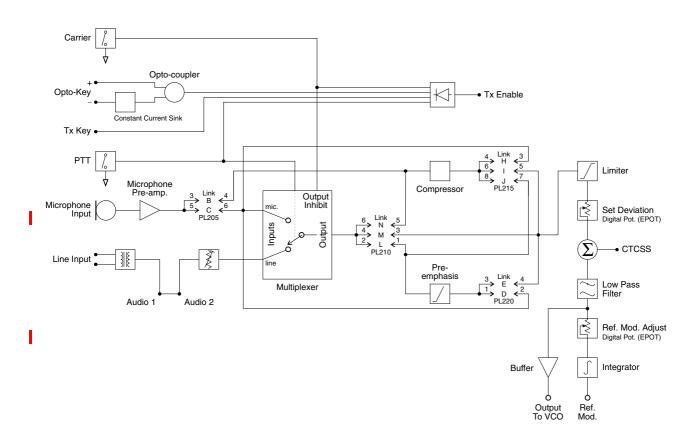
Figure 2.6 T836/837 Audio Processor Block Diagram
