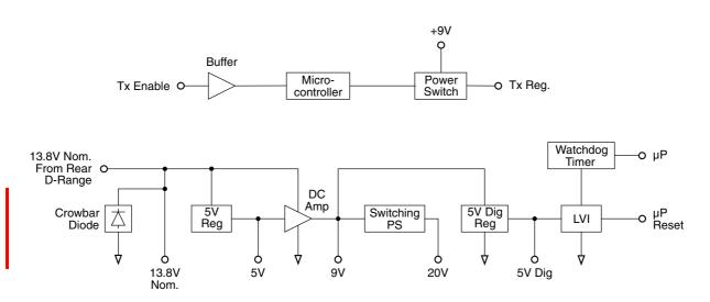
Figure 2.7 T836/837 Power Supply & Regulators Block Diagram
