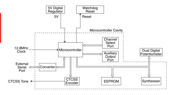
Figure 2.3 T836/837 Microcontroller Block Diagram
